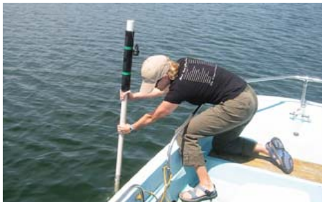
An integrated sampler is used to collect water samples for analysis.
