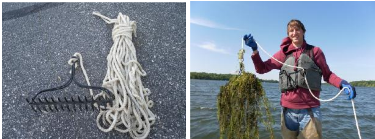
Figure 1. Double-headed, weighted garden rake, attached to a rope used to survey aquatic vegetation.
